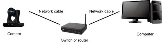
2. To connect directly through network cable, the IP address of the computer should be changed so that it is on the same network segment as the camera
